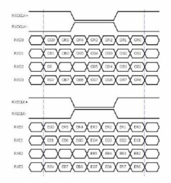
Note 1: R/G/B data 7:MSB, R/G/B data 0:LSB O = "Odd Pixel Data" E = "Even Pixel Data"
